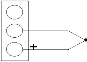
**TWO WIRE TRANSDUCER CONNECTIONS
