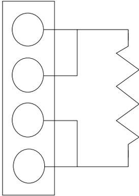
**THREE WIRE TRANSDUCER CONNECTIONS**
